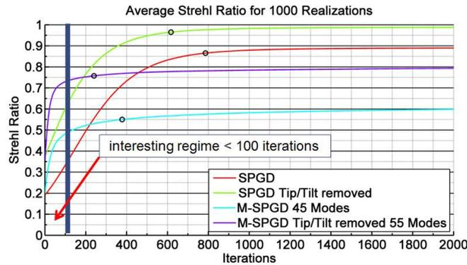
Fig. 1. Illustration of convergence of SPGD and M-SPGD algorithms. Black circles denote points on the curves where the quality metric, here the Strehl ratio, starts to change by less than  $10^{-4}$ . The blue vertical line denotes the region of less than 100 iterations which for practical reasons is the most interesting.
